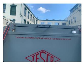
Next, lift the unit using the grill handle in the middle. The lid must be open to the maximum height of the gas struts.
