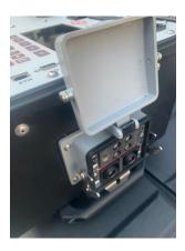
Put the Staubli connector of the PL4150 into the pins of the T4350. Note, the bottom two circular connectors need to be facing in the downwards position.
