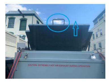
Unlatch the Staubli connector by pushing the metal lock in the upwards position. **NOTE:** You MUST have your opposite hand holding the connector tightly as it can fall off due to the force of gravity and damage the connector and or your vehicle.
