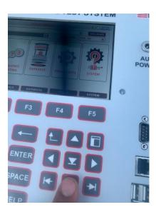
For manual mode testing select F1 on the keypad.
