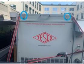
To unlatch, pop the bottom of the latch upwards
