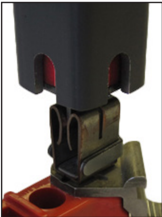
Meter socket with hot socket gap indicator testing before & after the socket safety clip is installed
