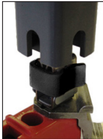
Meter socket with hot socket gap indicator testing before & after the socket safety clip is installed
