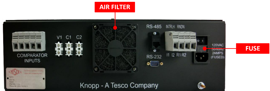
Figure 5.2. KATC-C2 Fuse and Air Filter location
