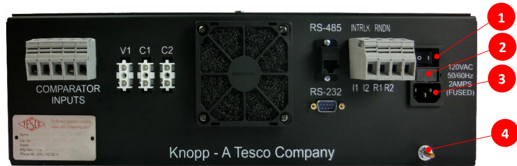
Figure 2.4. KATC-V2 Main Power Supply
