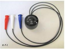
in time of the different voltage peaks of a multiphase supply. In addition, the Knopp Sequence Indicator enables one to make continuity tests. It is a valuable instrument in diverse fields involving polyphaser power apparatus, being employed by line and installation crews for public utility systems and industrial-plant electrical departments. It is, furthermore, helpful in the testing departments of public utility systems for laboratory and field testing.
