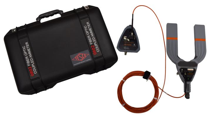
The TESCO Fiber Optic Coupled Ammeter was developed using current sensor technology. It is a two-piece, True RMS ammeter with a fiber optic link between the high voltage sensor and the readout at ground potential. The sensor is mounted on a hot-stick and slipped over a high voltage line.
