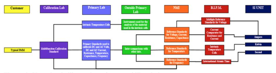
Figure 1: Very simple illustration of a traceability chain.
