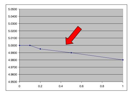
At 0.5Ohms of Burden the secondary current is still at 4.990A – Less than 0.3% change – Good CT! Initial Reading = 5Amps  $0.3\% \times 5A = 0.015A$ 5A - 0.015 = 4.985A
