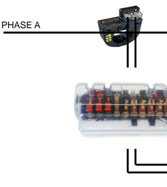
Some burden will always be present – junctions, meter coils, test switches, cables, etc.
