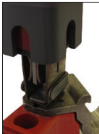
Red indication of a "bad" socket gap/loss of spring force.
